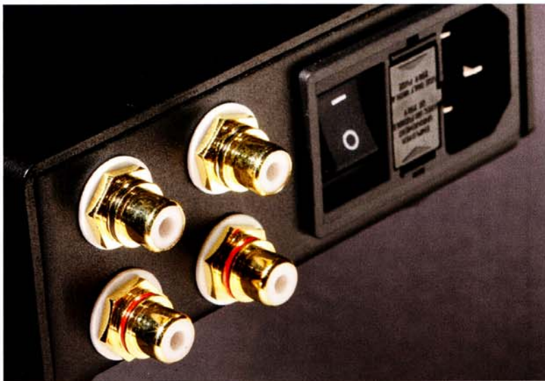
ABOVE: Not two inputs but a combination of L/R stereo input and variable preamp output, controlled off the same volume control as the two front headphone sockets
